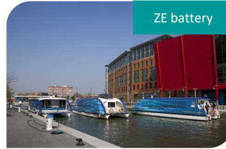
4 * Navettes Millénaire Paris - France 2*22 kW, 2*55 kWh, 75 pax
