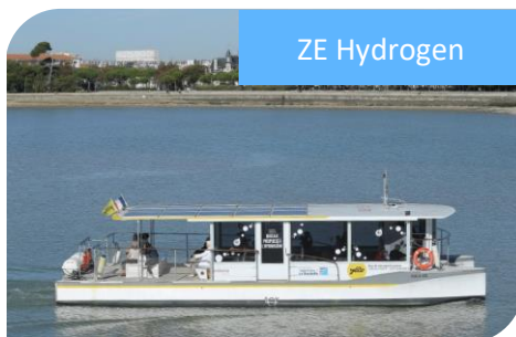
1 * Bus de Mer H2 La Rochelle - France 2*22 kW, 2*60 kWh, PAC 10kW, H2 7kg, 75 pax
