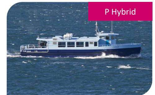
2 * EcoBatoBus Toulon - France 2*120 kW, Genset 340 kW ,2*85 kWh, 99 pax
