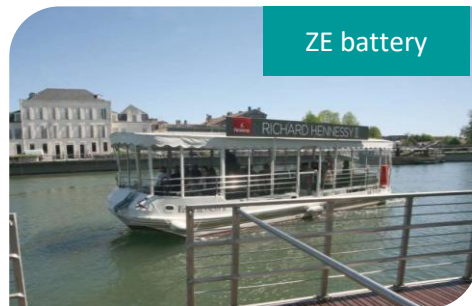
1 * Henessy II Cognac - France 15 kW, 30 kWh, 47 pax
