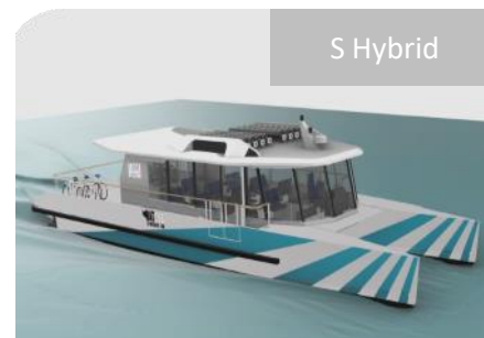
4 * WaterBus 60 - 2024 Bordeaux - France Hydrojet, 2*176 kWh, 60 pax
