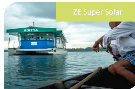
1 * Aditya India 2*20 kW, 2*25 kWh , 140 m 2 Solar pannels
