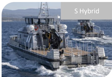
8 * CMM World 2*100 kW, 2*Genset 155 kW, 2*105 kWh
