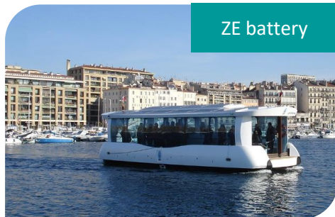
1 * Ferryboat Marseille - France 2 x 22 kW, 110 kWh, 45 pax
